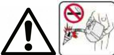
Handle fuel with care, it is highly flammable: Do not refuel machine while smoking, when machine is near an open flame or sparks, or when the engine is running. Stop the engine.
