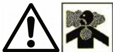
Engine exhaust fumes can cause sickness or death. If it is necessary to run an engine in an enclosed area, use an exhaust pipe extension to remove the fumes. Always try to work in a well ventilated area.
